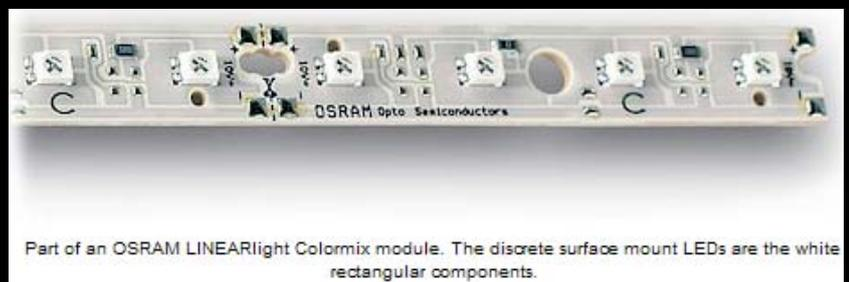
Part of an OSRAM LINEARlight Colormix module. The discrete surface mount LEDs are the white rectangular components.
