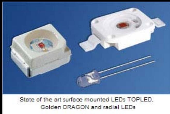
State of the art surface mounted LEDs TOPLED,
